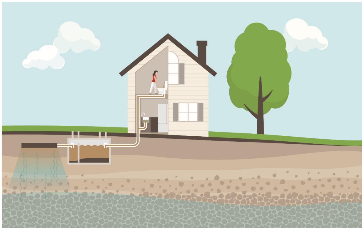
Figure 12. Conventional residential septic systems are currently designed to treat bacteria. Because they only treat 30–40% of nitrogen input, they can be a source of nitrogen pollution in the watershed | www.ourwatershed.ca .
