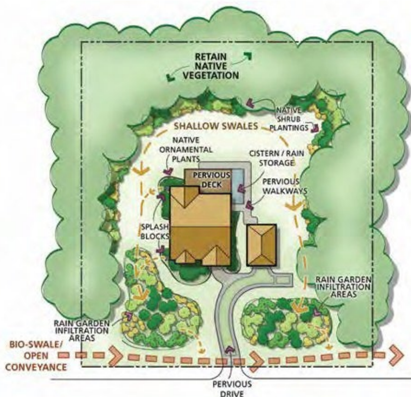
Figure 19. Green infrastructure techniques using Florida-Friendly Landscaping™ can capture and store water on residential lots | Puget Sound Partnership and WSU Extension.
