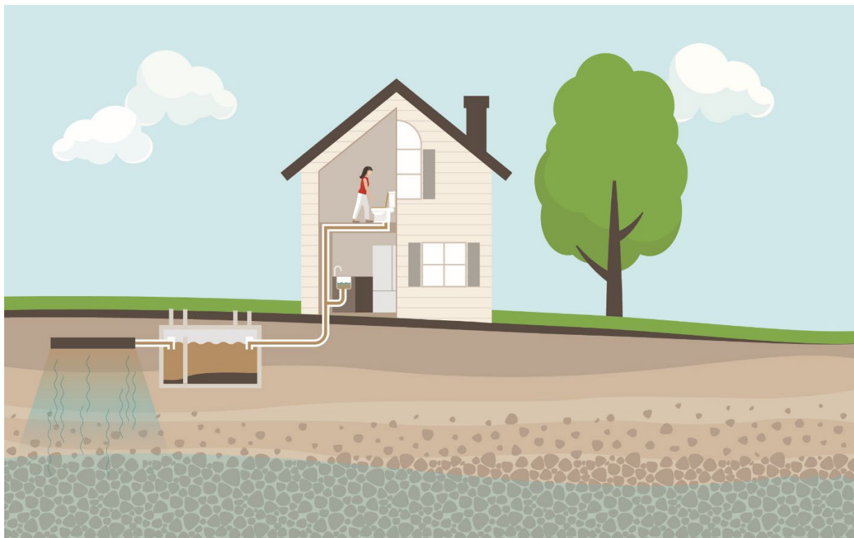
Figure 12. Conventional residential septic systems are currently designed to treat bacteria. Because they only treat 30–40% of nitrogen input (Toor et al. 2011), they can be a source of nitrogen pollution in the watershed | www.ourwatershed.ca .
