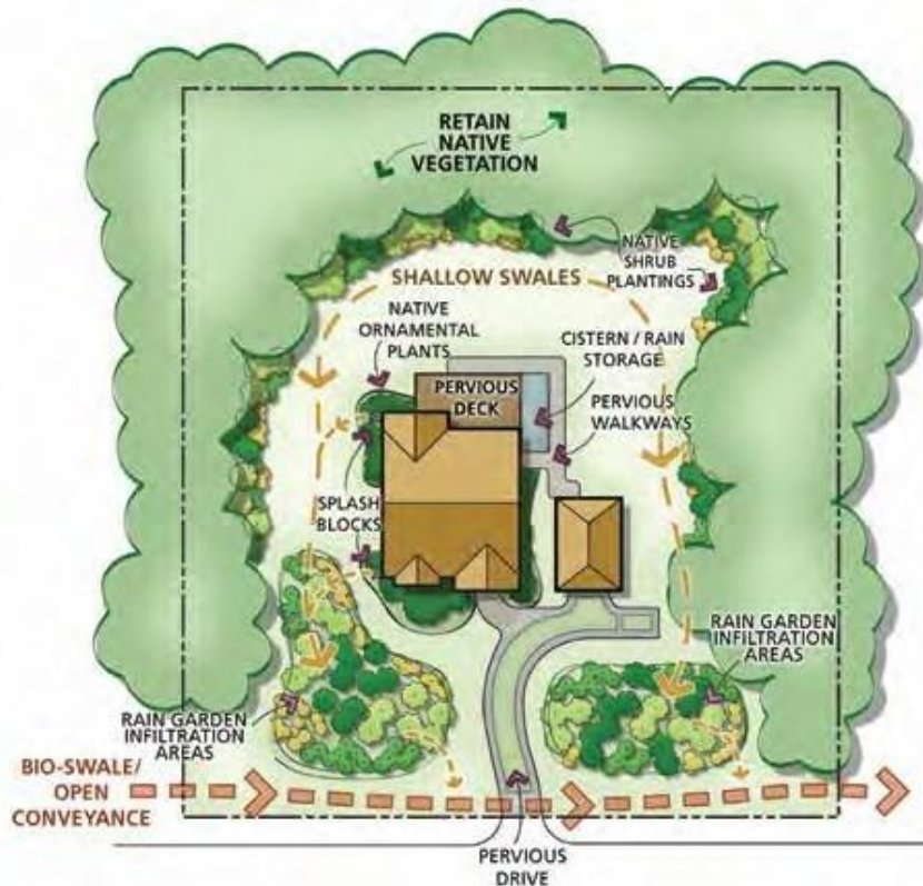
Figure 194. Green infrastructure techniques using Florida-Friendly Landscaping™ can capture and store water on residential lots. | Puget Sound Partnership and WSU Extension.
