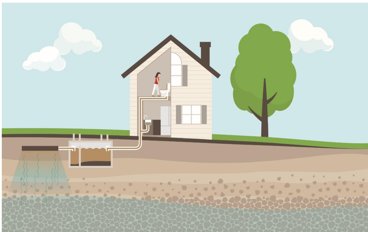
Figure 123. Conventional residential septic systems are currently designed to treat bacteria. Because they only treat 30–40% of nitrogen input, they can be a source of nitrogen pollution in the watershed | www.ourwatershed.ca .
