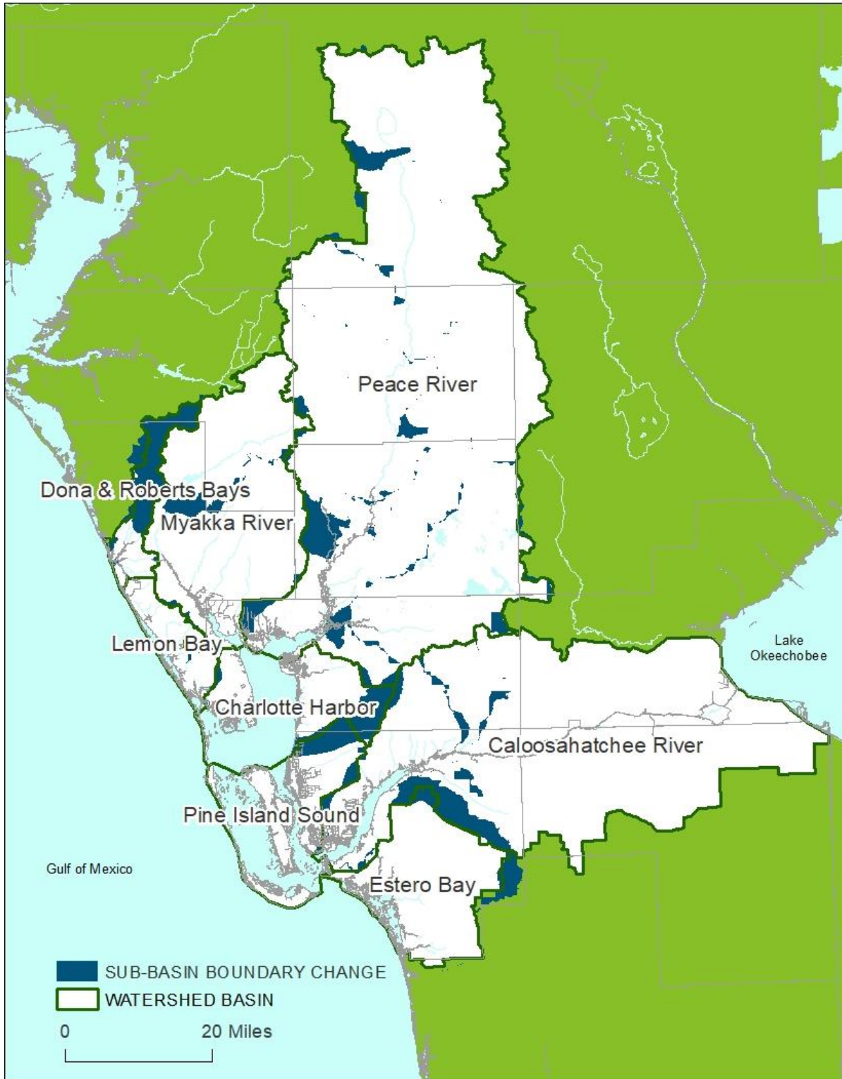
Figure 15. Historically, drainage projects to dry the land for agriculture and urban development rerouted surface water via canals to the closest waterbody, resulting in hydrologic shifts to the historical boundaries of watersheds and their sub-basins | CHNEP 2013.
